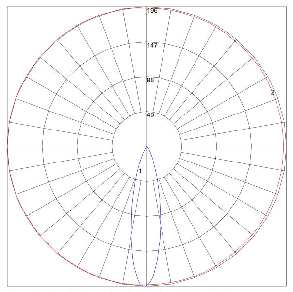
Maximum Candela = 196 Located At Horizontal Angle = 180, Vertical Angle = 1 # 1 - Vertical Plane Through Horizontal Angles (180 - 0) (Through Max. Cd.) # 2 - Horizontal Cone Through Vertical Angle (1) (Through Max. Cd.)
