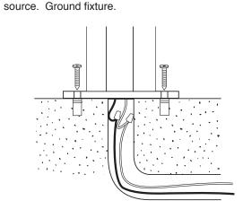
**4.** Use 1/4-20 flat head screws to bolt fixture to concrete anchors. Provide 24 volt AC voltage to LED light
