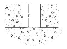
2. Run low-voltage wires into center of hole from 12V approved UL listed landscape transformer
