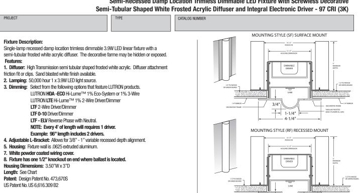
NOTE: This fixture is NON-IC. If fixture is installed in an insulated space, installation must be held back 3" from contact with fixture. Please check your local electrical and building codes.
